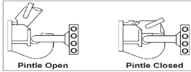
4. See the coupler instructions for details of placing the pintle in the “open” position.
